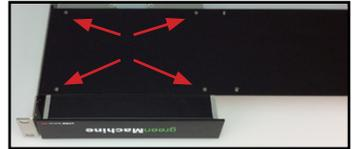
**Step 3:** Turn both the greenMachine modules upside down and place them next to each other. Remove the 4x feet from the bottom of each of greenMachine. Set the eight screws together with the feet aside for possible later use.
