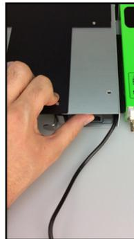
**Note:** The power supply should slide into the power supply mount without resistance. If not, then remove the power supply and make sure the power cord is positioned correctly.
