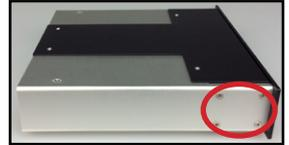
**Step 7:** Remove the power supply mounts.
