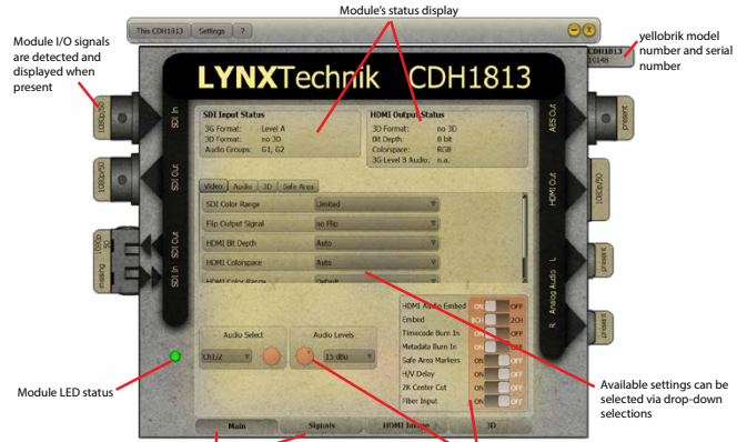
Access to additional information and screen displays are provided using the buttons along the bottom of the GUI
