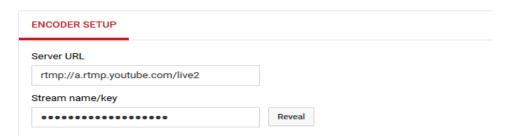
3. Insert the above information in the PEC 1864 as shown in the picture on the right side and the PEC 1864 is ready to stream.
