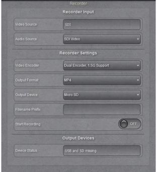
**Note:** The recording process can be started and stopped in the Web UI using this on/off switch or via the record button at the left side of the module.
