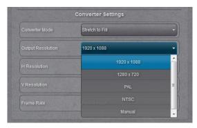
If one of the converter modes is selected, the output resolution can be set: 1920x1088, 1280x720, NTSC, PAL, Manual (Default = 1920x1088)
