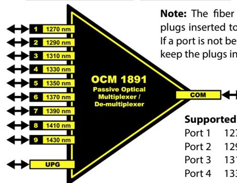
**Note:** The fiber connection ports will have plugs inserted to prevent dirt contamination. If a port is not being used we recommend you keep the plugs in place.
