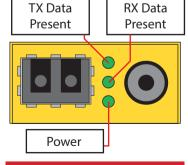
WARNING: Module laser is active as soon as power is connected, regardless of LED indication
