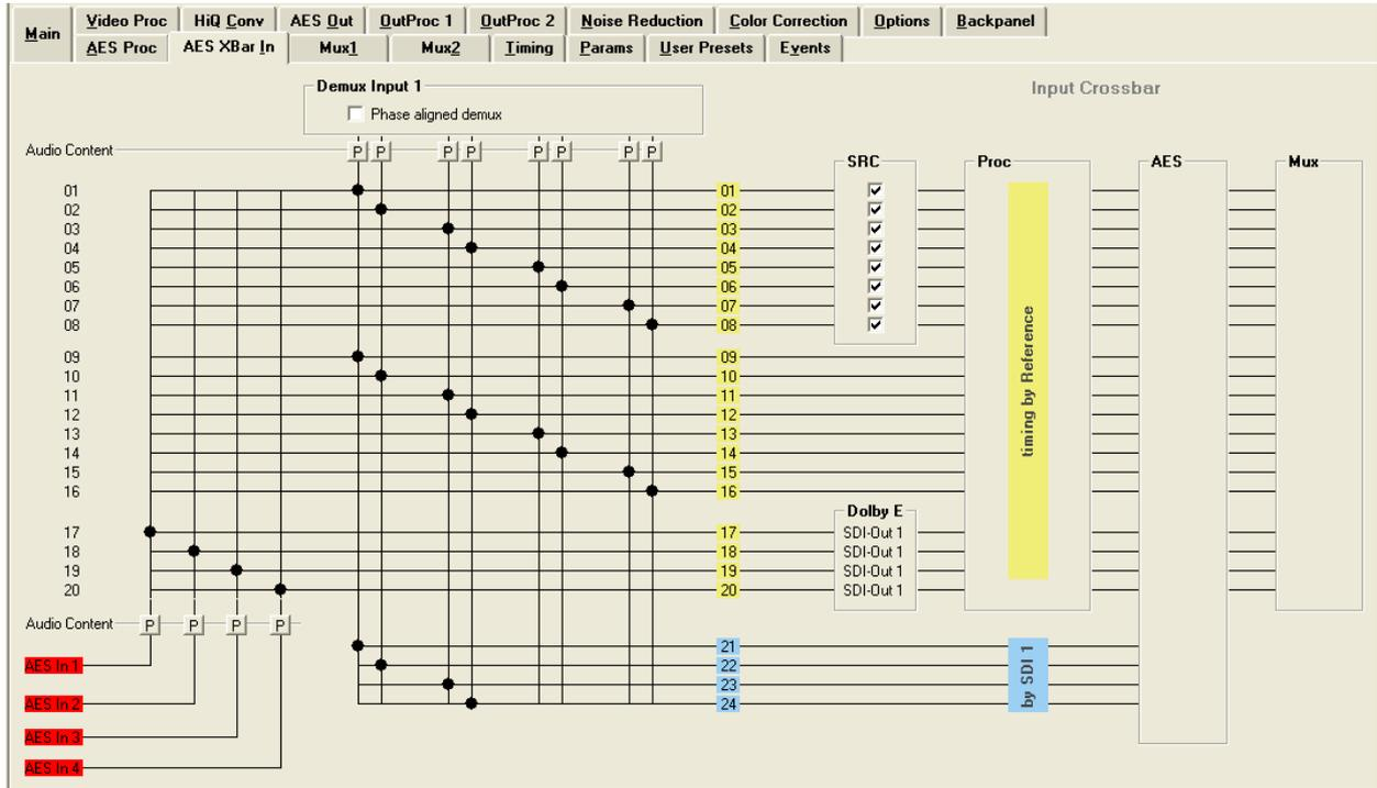
The crossbar arrangement is simple; the inputs from the de-embedder come in from the top. The external AES inputs come in from the bottom. All audio inputs are the vertical component of the crossbar. The audio pathways out of the crossbar are horizontal. Routing an AES pair is achieved by clicking on the cross point with the mouse cursor.
