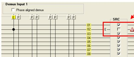
Here you can see DolbyE has been routed into audio Pathway 1, channel 2. The module has inserted the warning symbol.
