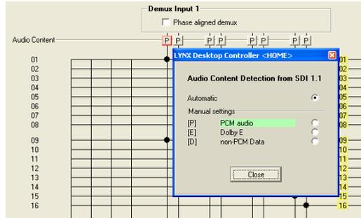
The default setting is always automatic, as seen above and for this first input you can see it has detected PCM audio.
