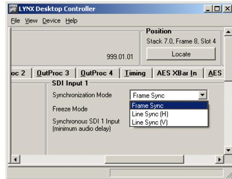
**Line Sync (H):** In case of clock synchronized signals the Line synchronizer H mode can be activated to achieve minimum delay. The input signal is buffered for 1 line to correct timing differences within 1 line
