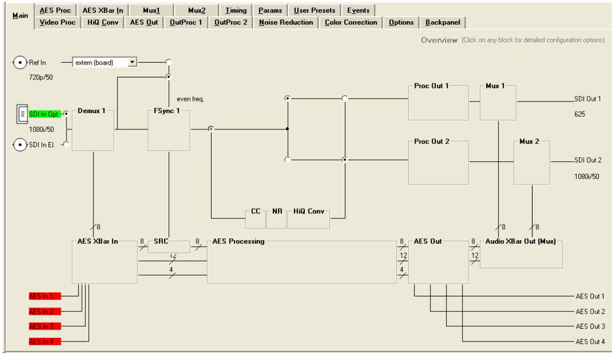
The primary purpose of this screen is to show the overall signal flow through the module and allow easy navigation to other areas. Input standards and formats are auto detected and displayed in the GUI. Parameters will be annunciated in different colors to show status (green = good, red = problem, yellow = caution etc).
