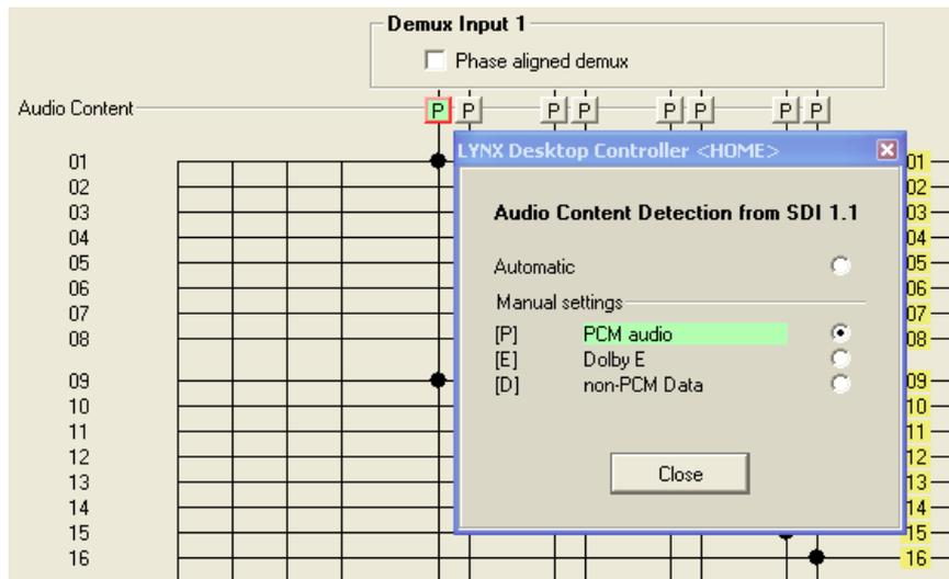
In this case you can see input 1 has been manually configured for PCM audio, and it is highlighted green to indicate it is a manual selection, and there is no conflict. (a box with a letter inside which is not green indicates this channel is configured for automatic detection)
