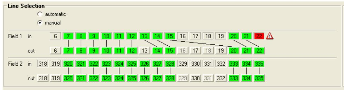
The encoder always tries to map the same input line to output line, in our example above line 17 and 19 are not used on the output as they were not used in the input. Clicking on these line numbers would activate their use in the output.
