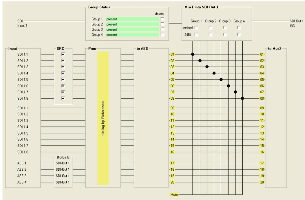
All of the internal audio from pathways 1, 2 and 3 are made available as inputs to each embedder. The embedder can be seen at the top of the GUI and it’s possible to quickly disable or enable an individual AES “Group” using the checkbox provided.
