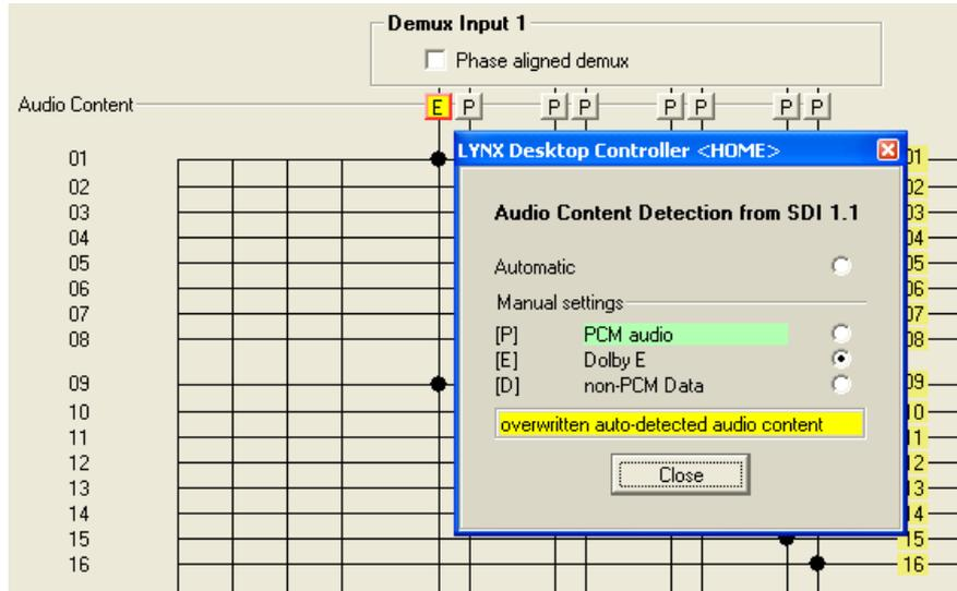
Here you can see the conflict is flagged by turning the box yellow. This is indicating the channel is manually preset for Dolby E, but the audio format is in conflict with this setting, in this case PCM audio. **Note.** *Even though there is a conflict the actual audio content is passed through the system – i.e. it is not blocked.*
