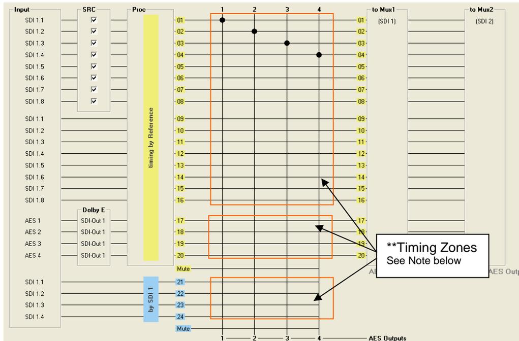
All inputs to the crossbar are shown horizontally and the 4 x External AES outputs are shown at the bottom of the screen. Selecting a cross point will route the required signal to the selected AES output. There is also a “mute” function for each AES output if required.
