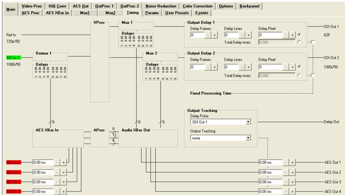
The video delay can be adjusted for the two SDI outputs independently.
