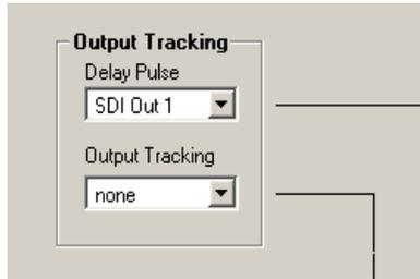
Use the drop down list provided to link the four external AES outputs to one SDI output channel auto tracking delay value.
