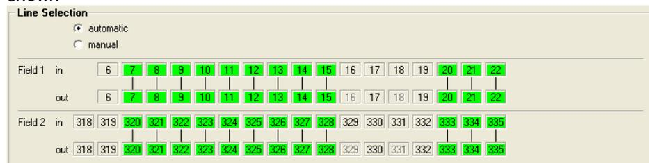
In automatic mode the output line numbers equal the input line numbers. Manual mode has to be selected to change the output line numbers.
