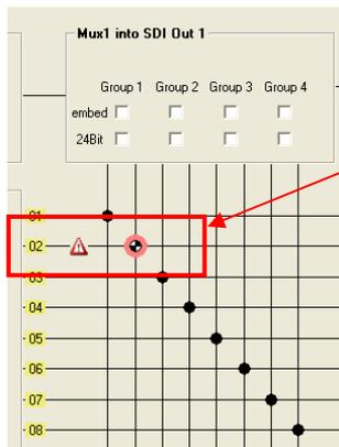
Here you can see the highlighted cross-point has been manually changed from its default settings. The warning symbol clearly indicates there is a conflict with this cross-point setting for the audio signal present.
