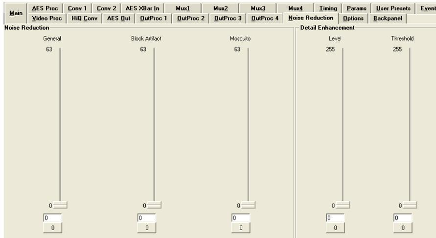
The adaptive noise reduction function processes the input data in either progressive or interlaced format. Application of noise reduction to noisy interlaced signals can optimize de-interlacer performance.
