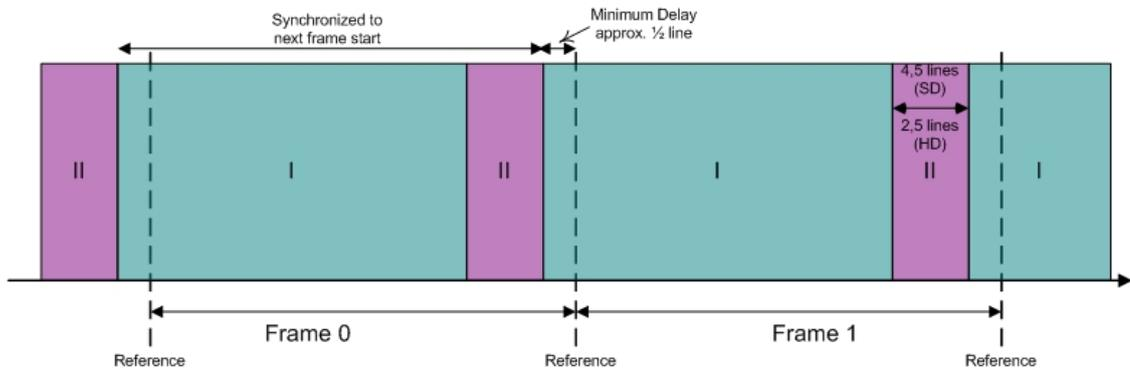
For distortion free switching in front of the P VD 5806, e.g. in a router, all signals have to be in area "I" or all signals in area "II".
