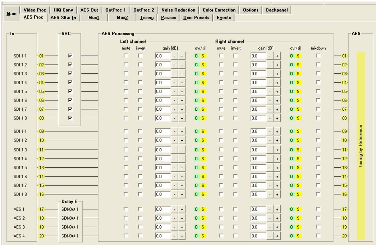
**Note:** If any Dolby E signal or other Audio data is passed through the processing stage, the processing will be deactivated, so the audio data will not be modified (controls will be greyed out). Settings will be set back to the original value if PCM audio will be switched to the same path.
