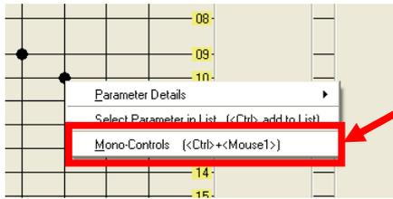
Select "Mono Controls" from this small submenu and a new mini cross point control box is displayed
