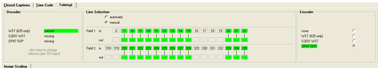
A pre-selection can be set by clicking on the text at the bottom of the decoder window. This will open the Video Proc tab, where the pre-selection can be set for the two inputs.
