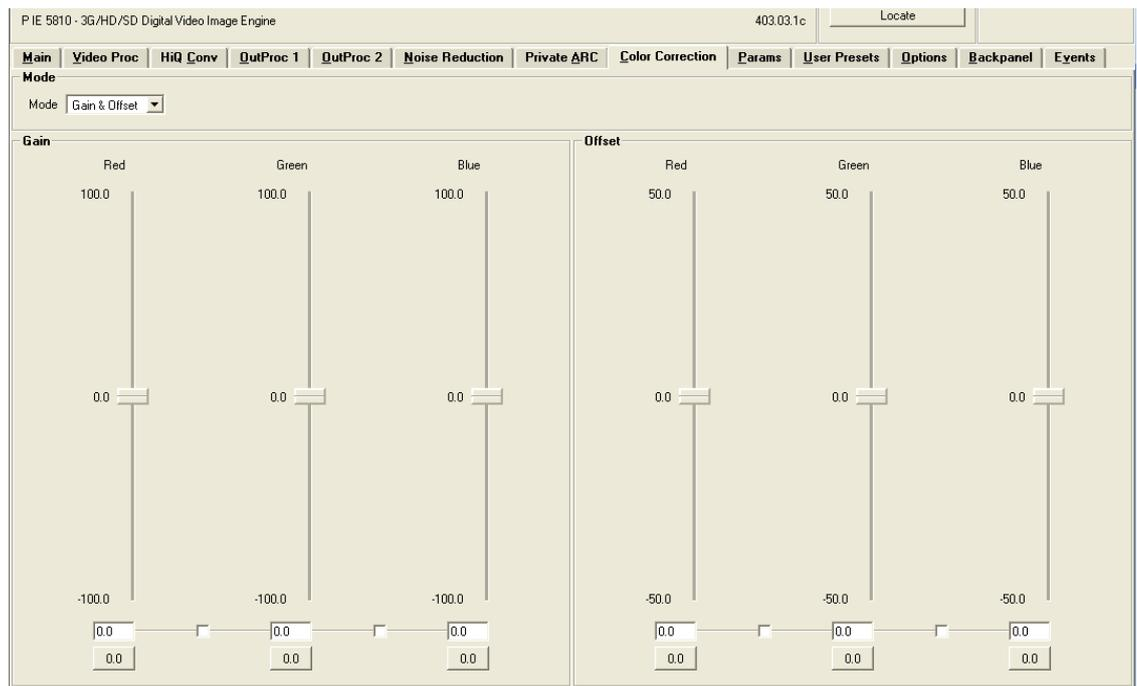
Gain amplifies the signal until it is clipped. Offset lifts the black level of the complete signal without impact on the gain.
