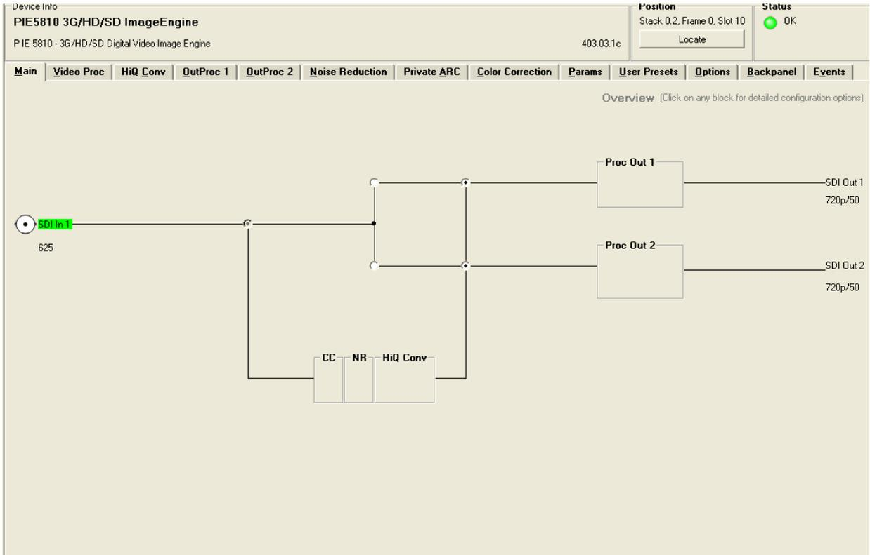
The primary purpose of this screen is to show the overall signal flow through the module and allow easy navigation to other areas. Input standards and formats are auto detected and displayed in the GUI. Parameters will be annunciated in different colors to show status (green = good, red = problem, yellow = caution etc).
