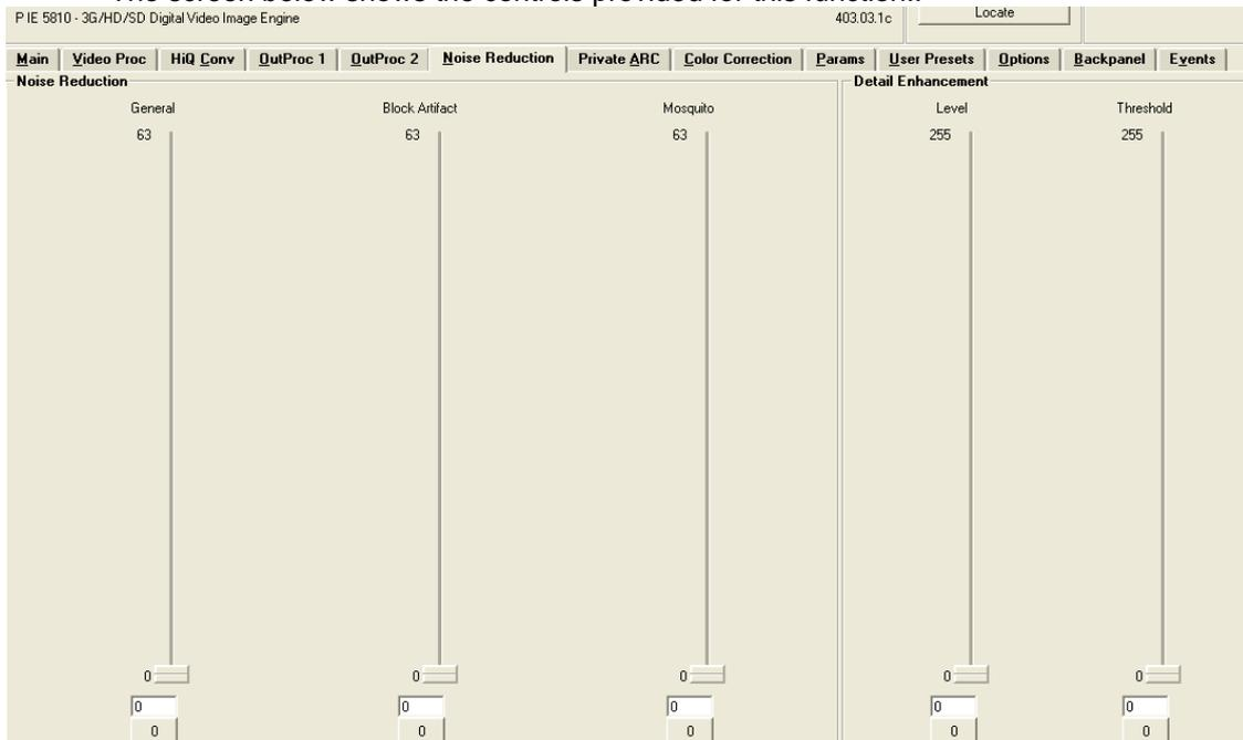
The adaptive noise reduction function processes the input data in either progressive or interlaced format. Application of noise reduction to noisy interlaced signals can optimize de-interlacer performance.
