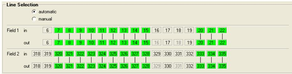
In automatic mode the output line numbers equal the input line numbers. Manual mode has to be selected to change the output line numbers.
