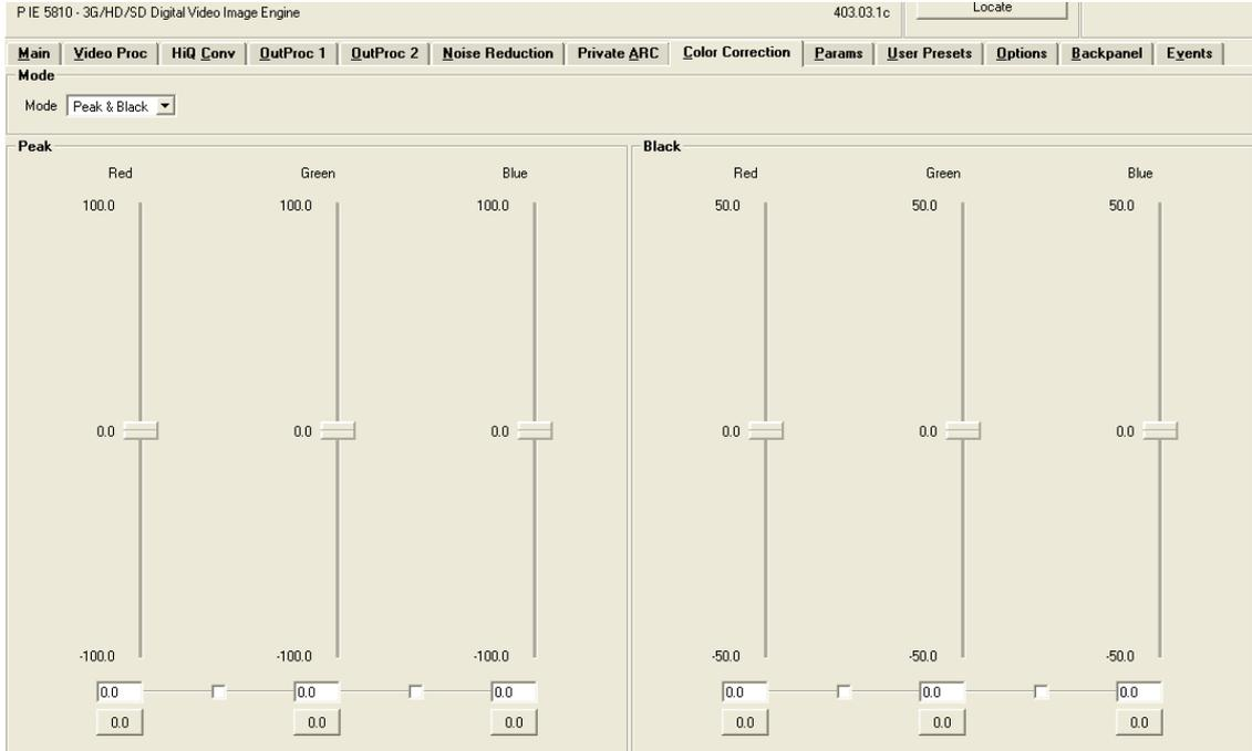
Peak sets the white level of the signal without changing the black level. Black sets the black level of the signal without changing the white (peak) level.
