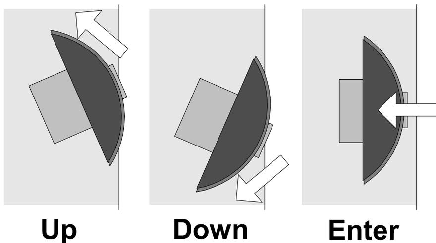
Figure 4 – Switch Operation
