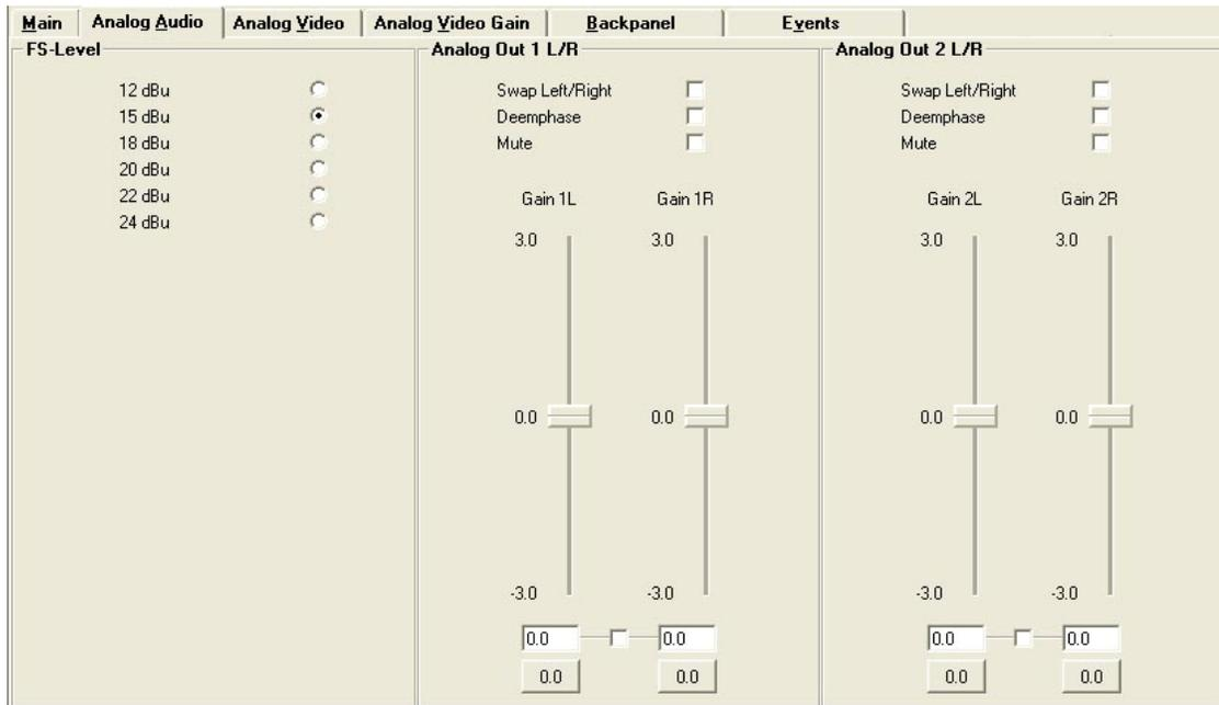
This GUI screen provides access to all the analog audio adjustments and settings. The gain adjustment provided is +/- 3dB from the selected Full Scale Level (FS Level)
