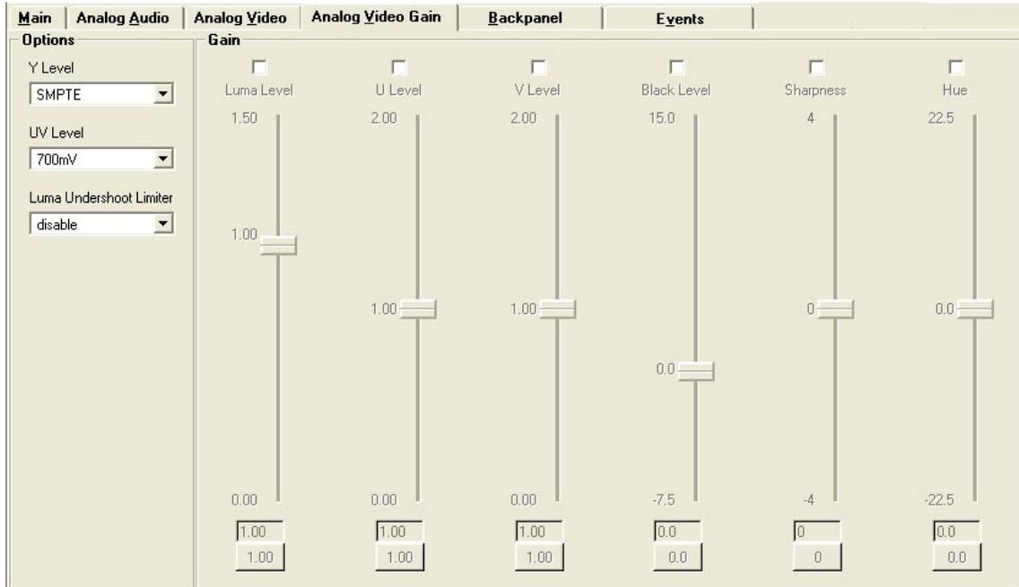
This GUI screen provides access to the internal video processing amplifier where gain levels can be adjusted and set. Default is a null setting for all adjustments.
